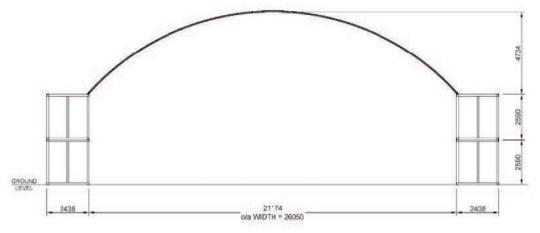
Rapid-Span structures are constructed as an arched roof fixed to shipping containers, steel columns, concrete walls or the side wall of existing structures.
