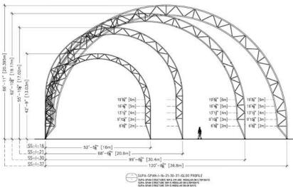
Supa-Span Igloo profile is designed with a curved frame assembly ranging from 16m/53ft - 30m/100ft standard span. Larger spans can be engineered to meet your exact needs.
