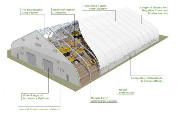
The TFS 380 Series is an alloy framed structure, pre-engineered to the highest quality standards, in addition to being designed to suit a wide range of applications including Aviation, Mining & Energy, Sport & Recreation, Industrial and Remediation.
